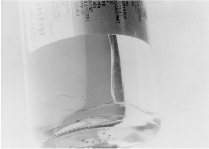
Figure 1: Cracked borosilicate vial of contaminated human albumin which upon injection resulted in blood stream infections for patients 4 .
