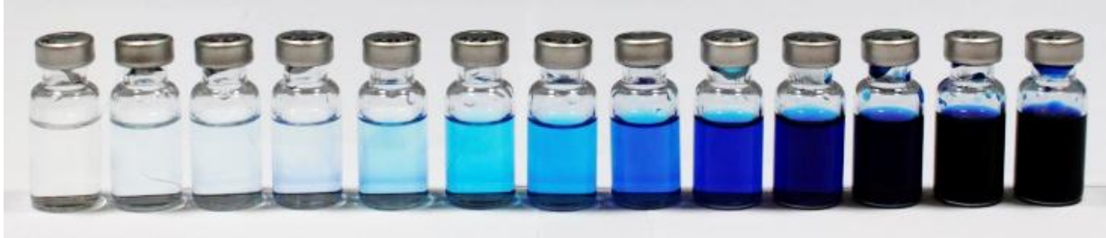
Figure 10: Positive control population for semi-quantitative comparison of dye ingress tests. The vial set shows (from left to right) a process blank (no methylene blue) and serial dilutions of methylene blue dye from 0.000049% to 0.1%.
