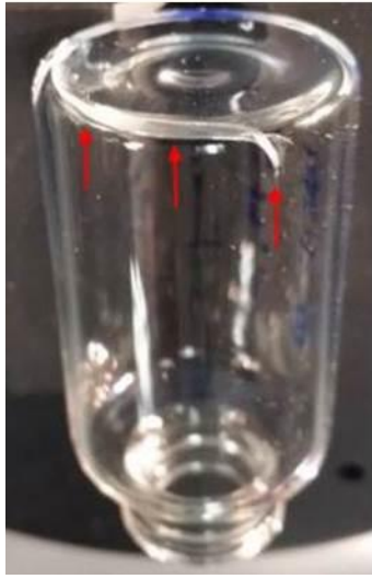
Figure 8: a) Field returned borosilicate vials that experienced a lensing crack that propagated up the sidewall from additional applied stress but did not break the vial. b) Optical microscopy image of two vials from controlled lab experiments that replicated these lensing cracks.
