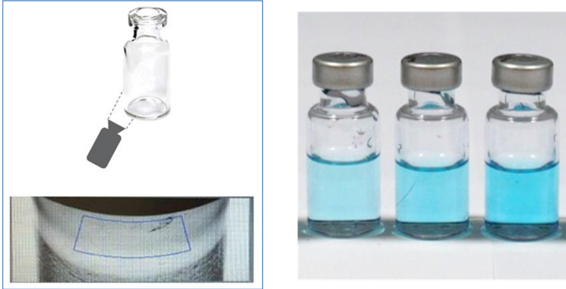
Figure 14: a) At left, an illustration shows the orientation of a state-of-the-art automated inspection camera designed to reject vials with cracks in the lensing crack region, with an example photo at bottom. b) At right, a photo of vials that were accepted as good by the automated inspection system shows that they clearly failed the dye ingress testing as indicated by the presence of blue dye.
