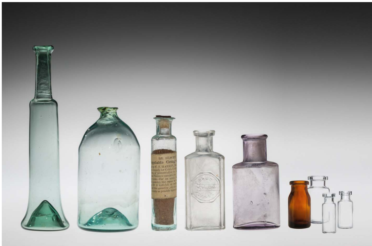
Figure 3: Evolution of pharmaceutical container shape, size, color and glass composition from 1600s through today. From left to right: (a) manually free-blown soda-lime bottle c1600-1699, (b) manually mold-blown soda-lime bottle c1700-1799, (c) manually mold-blown soda-lime vial c1840-1860, (d) manually mold-blown soda-lime bottle c1865-1915, (e) semi-automatically mold blown soda-lime bottle c1880-1920, and (f) borosilicate vials: mold blown amber, tubular converted clear c2013-2016. Objects (a)-(e) from the collection of the Corning Museum of Glass, Corning, NY.
