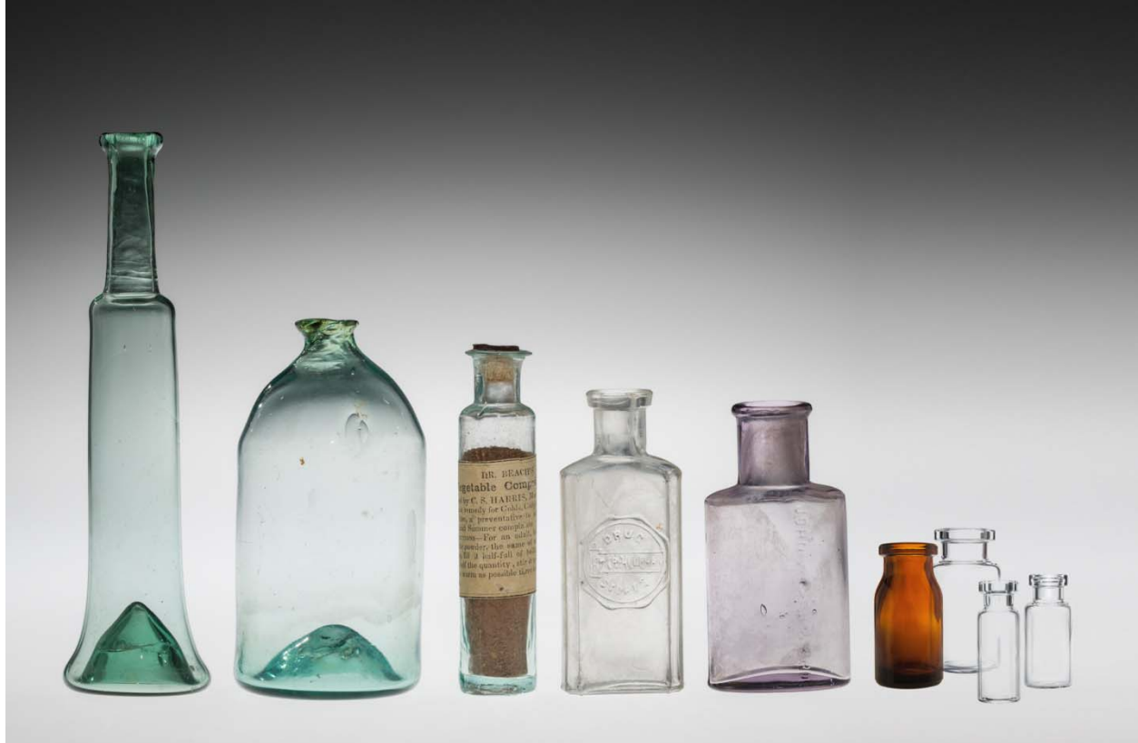
Figure 3: Evolution of pharmaceutical container shape, size, color and glass composition from 1600s through today. From left to right: (a) manually free-blown soda-lime bottle c1600-1699, (b) manually mold-blown soda-lime bottle c1700-1799, (c) manually mold-blown soda-lime vial c1840-1860, (d) manually mold-blown soda-lime bottle c1865-1915, (e) semi-automatically mold blown soda-lime bottle c1880-1920, and (f) borosilicate vials: mold blown amber, tubular converted clear c2013-2016. Objects (a)-(e) from the collection of the Corning Museum of Glass, Corning, NY.
